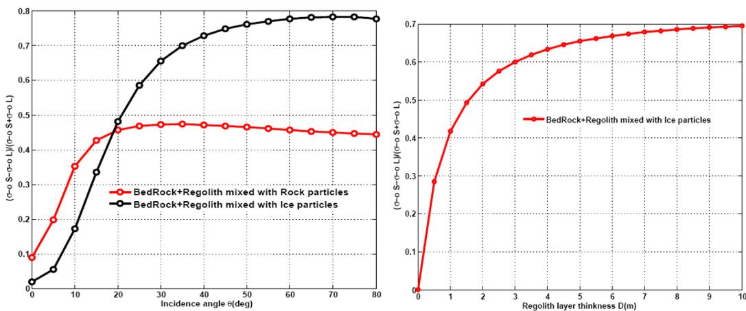
Fig 2: a) Variation of LPDI as a function of incidence angle and b) regolith layer thickness
