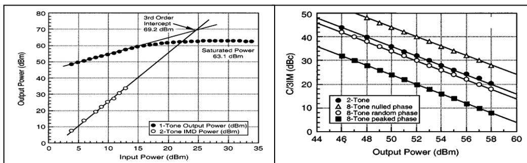
**Fig.2: (a) 1-tone output power & 2-tone I/M power vs input power, (b) C/3IM vs output power**
